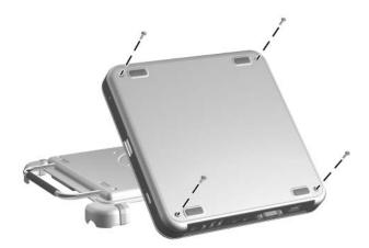
Removing the Top Case Screws
